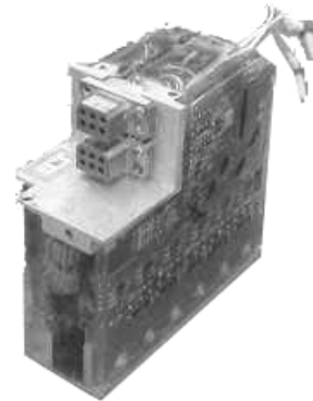
Fig. 8 One sub-module of FE modulator
